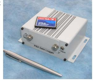
Applications include simultaneous logging of navigation with sensor data (fathometer, gyrocompass, etc.) and remote unattended data logging. All operating parameters, including com port baud rate and message definitions, are stored on the Compact Flash card. Data can be easily read from the Compact Flash card on any Windows equipped PC using a Compact Flash card reader.
